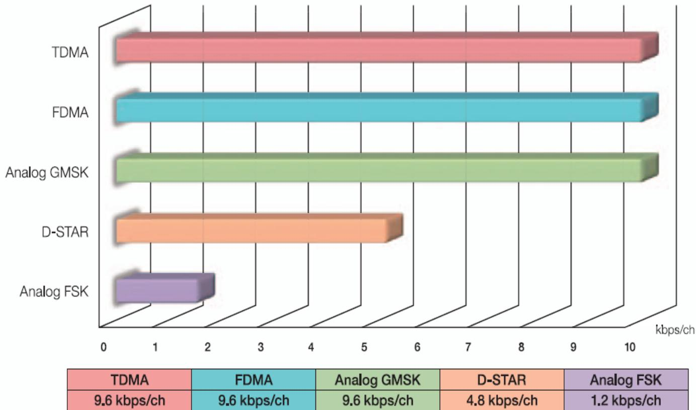
Fig. 7 Comparison of the data transferring speed
