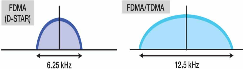
Fig. 8 Comparison of the occupied bandwidth
